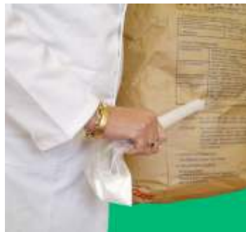
Insert the sampler through the side of the sack.
