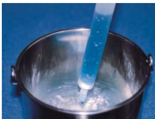
Discharge - Turn valve so that sample can be deposited into collection container
