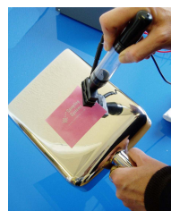
3. Place the Etching Mask and apply the etching fluid using the Electrolyte Applicator
