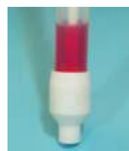
Sampler Tip Seal arrangement prevents sample from dripping
