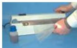
Cut the lay-flat tubing to length & seal one end
